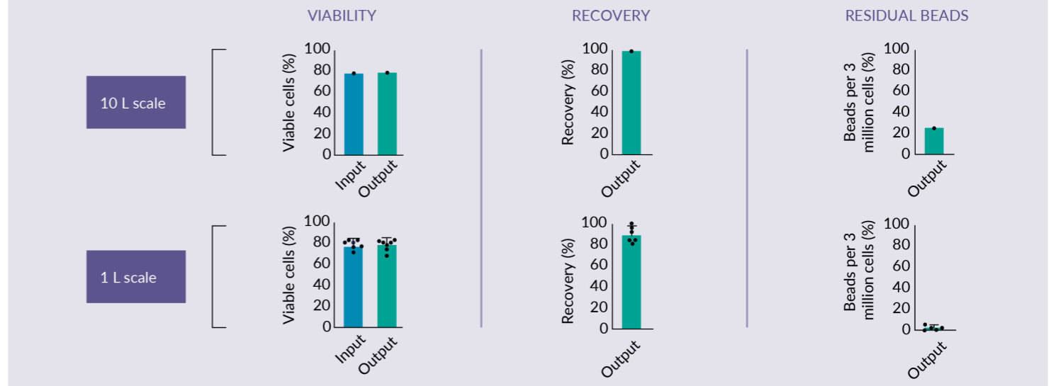
Figure 2. Viability, recovery, and residual beads after the bead removal process on the CTS DynaCollect at 1 L and 10 L scales.
